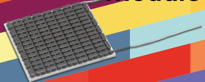
**Thermoelectric module (L×W = 40 mm × 40 mm) with dices size 1.4 mm × 1.4 mm × 1.6 mm (without upper substrate) with electrodeposited coating of all conductive parts: side surfaces of thermoelectric dices, copper contact pads atop, copper interconnection lead wires on lower substrate and solder surfaces between them. Temperature difference between hot and cold sides for module for cooling is from -80 °C to +100 °C; and for module for generation is from 20 °C to 280 °C**
